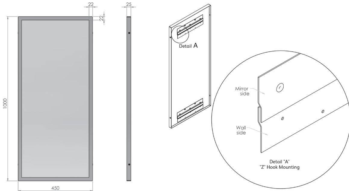
1. Using the integrated “Z-hook” mounting brackets, locate height on wall and mark fixing holes, ensuring unit is level and even.
