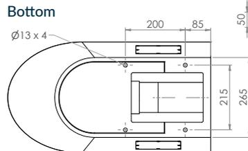
**Please Note: S trap pan is supplied with a separate pan bend. Set out dimension 130mm + or - 5mm.**
