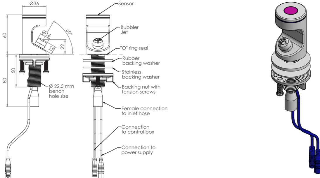
1. Remove the stainless steel backing nut, stainless steel washer and rubber washer . Ensure the rubber "O" ring in the base stays in place.
