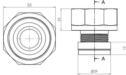
**URNNW-2:** Chrome Plated Sparge Adaptor. 50mm FI BSP to 25mm BSP Reducer
