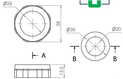
**URNNW-1:** This sparge adaptor is chrome plated and reduces from a 40mm thread to a 20mm or 25mm sparge pipe
