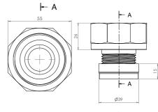
**URNNW-2:** Chrome Plated Sparge Adaptor. 50mm FI BSP to 25mm BSP Reducer
