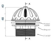
**URNPG:** Suits existing slab urinal outlets and replaces damaged or lost grates
