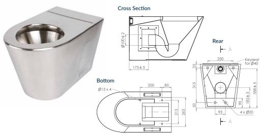
Please Note: S trap pan is supplied with a separate pan bend. Set out dimension 130mm + or - 5mm.
