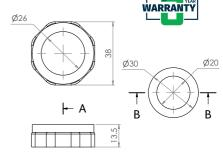
**URNNW-1:** This sparge adaptor is chrome plated and reduces from a 40mm thread to a 20mm or 25mm sparge pipe
