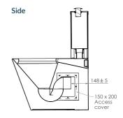
Please Note: S trap pan is supplied with a separate pan bend. Set out dimension 105mm + or - 5mm. Mini stop to be 150mm-350mm FFL and 100mm out from centre of pan.
