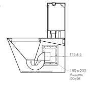
Please Note: S trap pan is supplied with a separate pan bend. Set out dimension 130mm + or - 5mm. Mini stop to be 150mm-350mm FFL and 100mm out from centre of pan.
