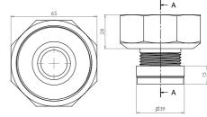
**URNNW-3:** This nut and washer is chrome plated. It accommodates 40mm sparge pipes
