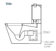
Please Note: S trap pan is supplied with a separate pan bend. Set out dimension 125mm + or - 5mm. Mini stop to be 150mm-350mm FFL and 100mm out from centre of pan.
