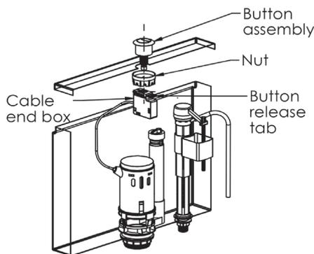
**Note:** This method will result in the buttons sitting about 20mm above the surface of the cistern. With the buttons fixed in their correct positions, re-connect the cable by pushing in the cable release tab and fitting the cable end box to the shaft of the button assembly.
